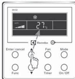
*Установка скорости вентилятора*
